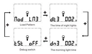
In load mode 3 (LM3), long press the+to enter the setting interface ,then short press+or — to set the parameters and save after long pressing + button.
